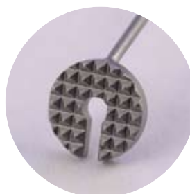
Fixation ring, diameter of working portion 7 mm, working portion made of stainless steel, diameter of titanium handle 5 mm, total length 80 mm
